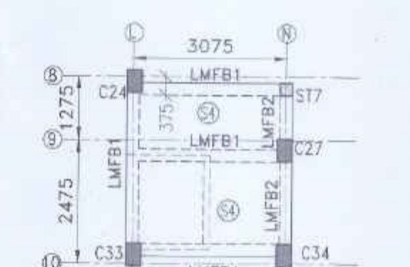
LMR FLOOR-2 BEAM AND SLAB LAYOUT PLAN AT LEVEL (+)16.450m. S4 MARKED SLABS ARE 150mm THICK. SCALE-1:100
